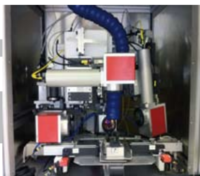
Four simultaneous marks on connecting rod by 4 galvano-heads
