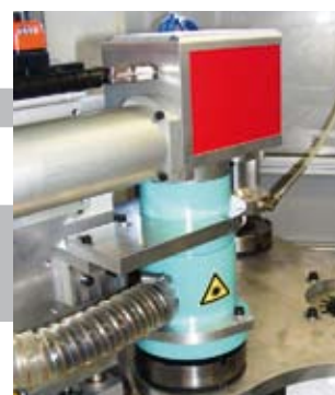
Laser Tunnel Protection
